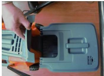
Press and hold in the safety Lock-Off Button located on the switch box.
