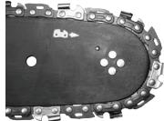
Move the guide bar (9) away from the driving chain wheel, so chain guiding links are placed in the guide bar groove.
