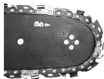
Move the guide bar (20) away from the driving chain wheel, so chain guiding links are placed in the guide bar groove.
