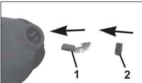
Remove and inspect the carbon brushes after periods of extended use. Replace them when they eventually wear down. The brushes should be kept clean and free to slide up and down in the holders. Both brushes should be replaced at the same time as a pair.
